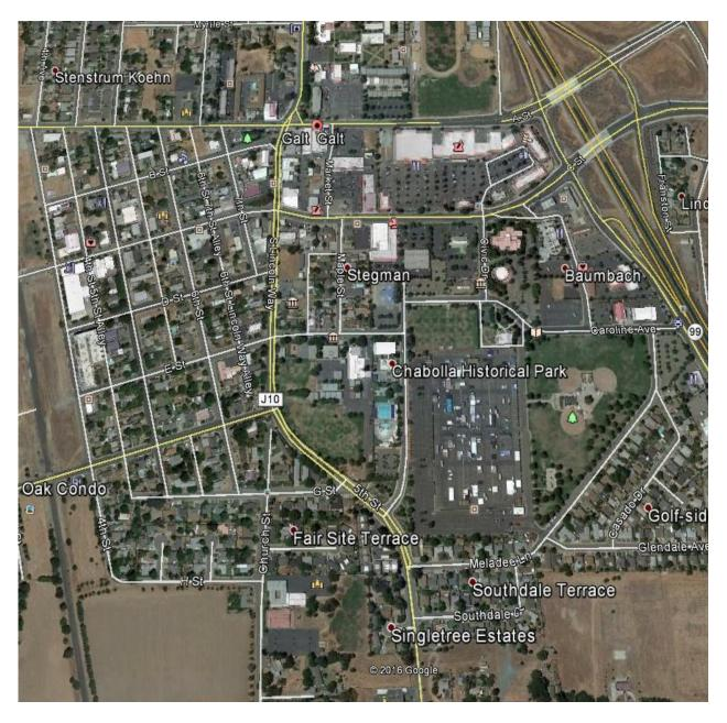
This Google Earth view shows the alignment through Galt. Notice the curve at the top of photo which eliminated the jog at "A" Street.
