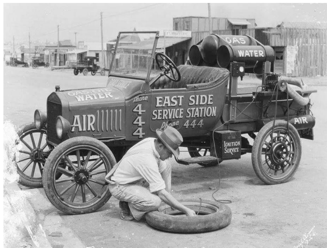
Independent Road Service Vehicle supplying gas, water, oil and tire repair with air provided by wheel driven compressor (attached to L/R wheel) operated when vehicle is in motion.
